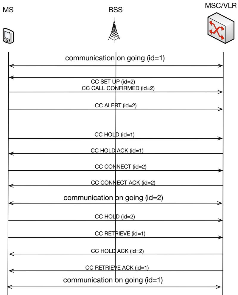
Figure 2: Radio procedure 2.
