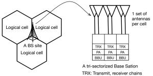
TRX: Transmit, receiver chains PA: Power amplifier BBU: Base band unit
