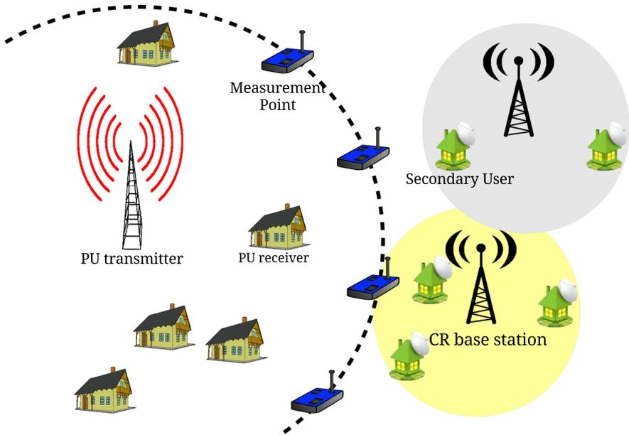
**Fig. 1** Network model: two CR operators serve clients
