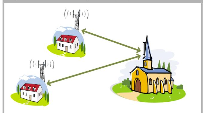
Fig. 2 Point-to-multipoint plus relay deployment to provide coverage in a shadow zone
