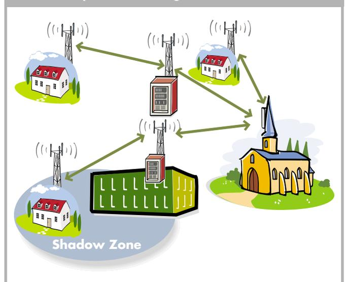
illustrated in *Figure 1*. However, the coverage is highly dependent on how the antenna is installed: clear path between the user's antenna and the access point, surrounding obstacles, and so on.
